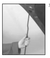
3. Lift the hood, release the hood prop from its retainer and put the hood prop into the slot in the hood marked "PROP ROD." Use the prop rod sleeve when handling the hood prop.
